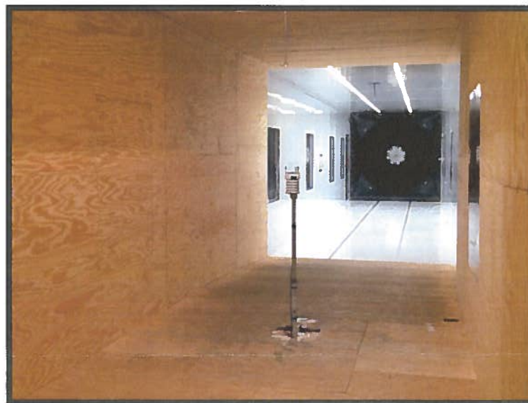
Photo of the wind tunnel setup. The cross-sectional area is 2.5 x 2.5 m.
